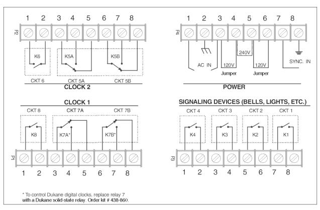
Figure 1-5 Master Clock Terminal Blocks
